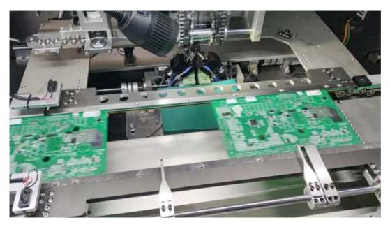
Centering gripper, keep component always alignment
